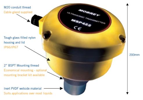
Once installed using the 2" thread, either directly to the vessel or on a suitable bracket above the liquid surface, 3 internal push buttons are used to programme the MSP422 with the tank depth and the range for the 4-20mA output.
