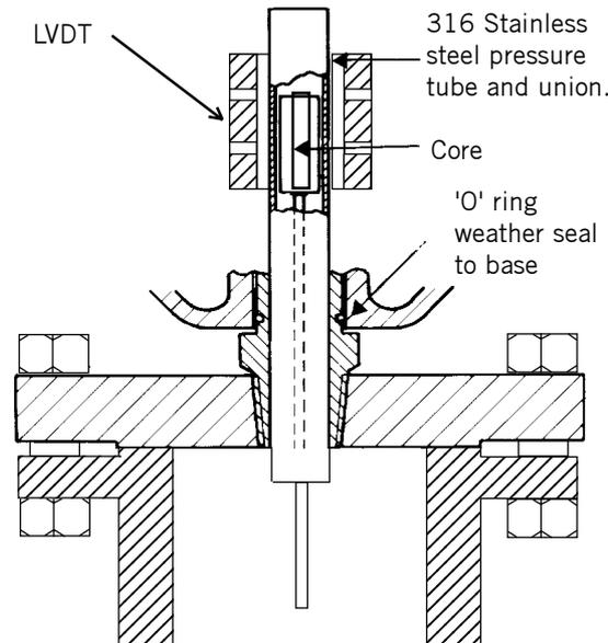
The displacer length is dictated by the operating range requested, and the diameter and weight are factory calculated to ensure the correct operating movement of the core in the head.
